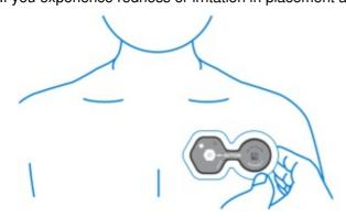
**REMOVE** adhesive from bottom of device. Follow steps 4 and 5 to put on a new adhesive and reapply BioSticker.
