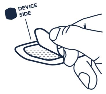
8. Place the **BIOBUTTON** on the exposed adhesive. Turn the device over and remove remaining adhesive backing.
