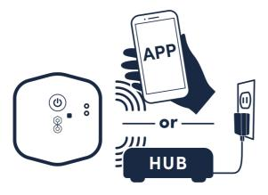
4. **CONFIRM BIOBUTTON ACTIVATION** by pressing the button and verifying that the light blinks **GREEN 4 TIMES.**
