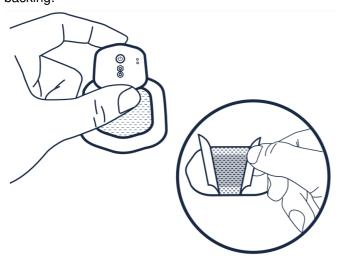
9. **ADHERE** the BioButton Rechargeable device to the upper left chest placement area. Apply pressure for 15 **SECONDS.**
