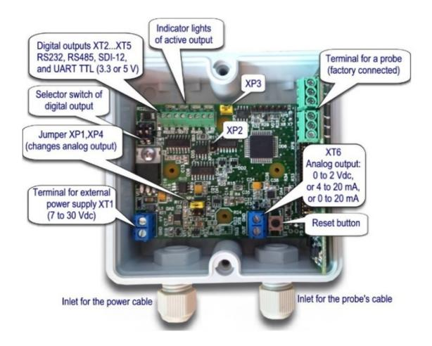
Select the desired type of analog output by appropriate position of the jumper XP1, XP4 as follows:
