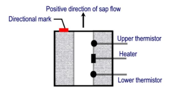
A spring loaded heater and a pair of bead thermistors are located inside the cylinder.
