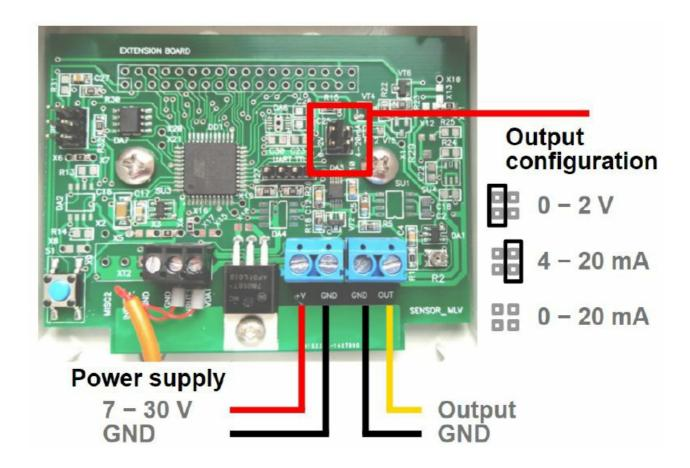
First, please choose a right output cable for connecting the sensor to a datalogger. The cable must be round with four wires. The maximal diameter of the cable is 6.5 mm. The cable length shall not exceed 10 m for 0 to 2 Vdc output (model LT-xM) and with about 1 km maximal length for 4 to 20 mA or 0 to 20 mA output (model LT-xMi).
