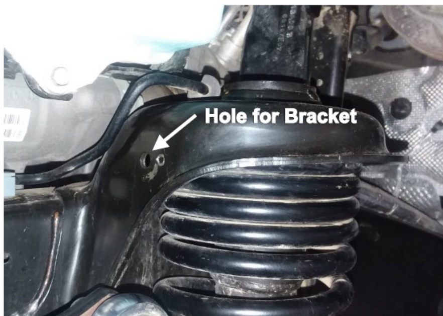
Figure 9 – Vehicle Left Side Spring Bucket
