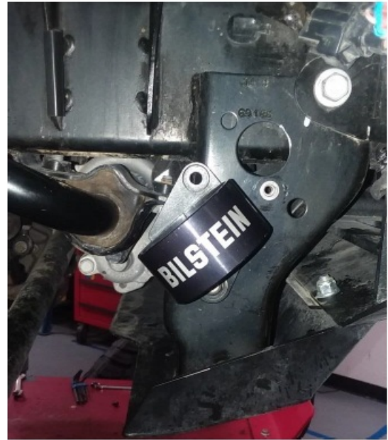
Figure 21 - Right Front Mount Assembly Tilted
