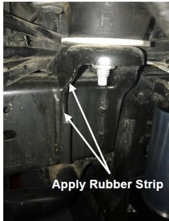
Figure 26 – Right Side Location for Rubber Strip
