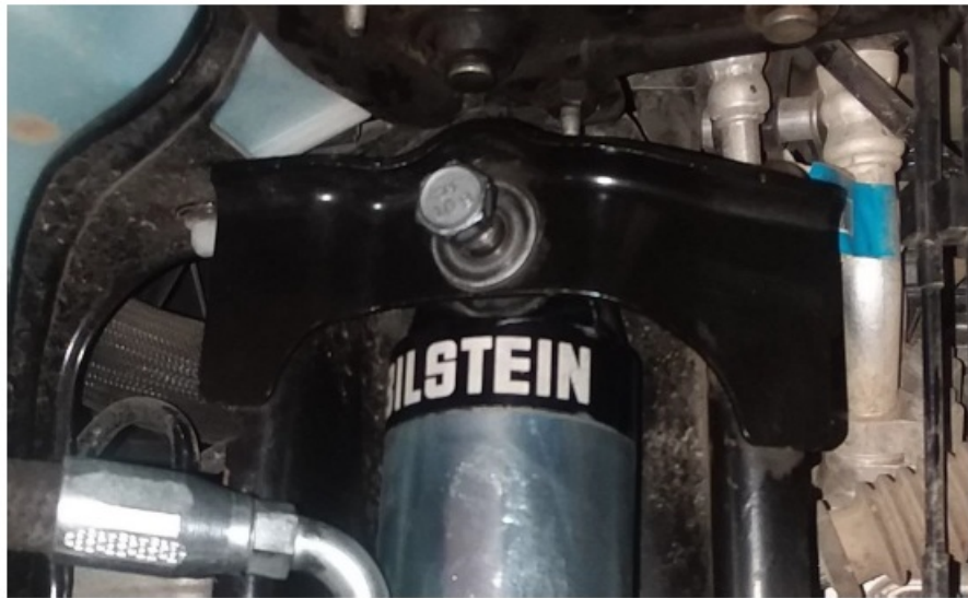
Figure 15 – Vehicle Left Side Upper Mount
