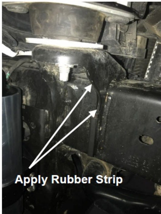
Figure 25 – Left Side Location for Rubber Strip
