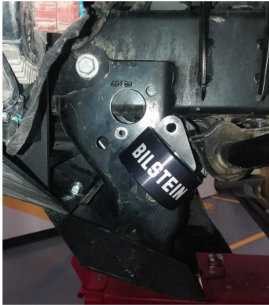
Figure 20 - Left Front Mount Assembly Tilted
