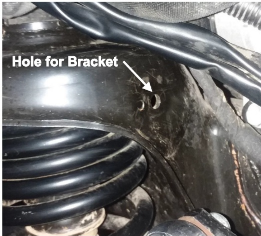
Figure 12 – Vehicle Right Side Spring Bucket
