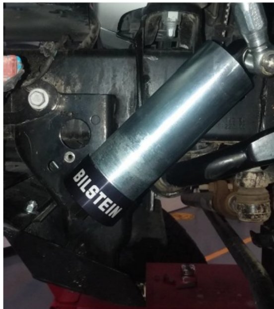
Figure 22 - Left Front Reservoir Slide Into Mount
