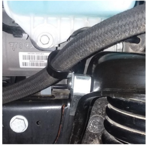
Figure 28 – Left Reservoir Hose Installed (Side View)
