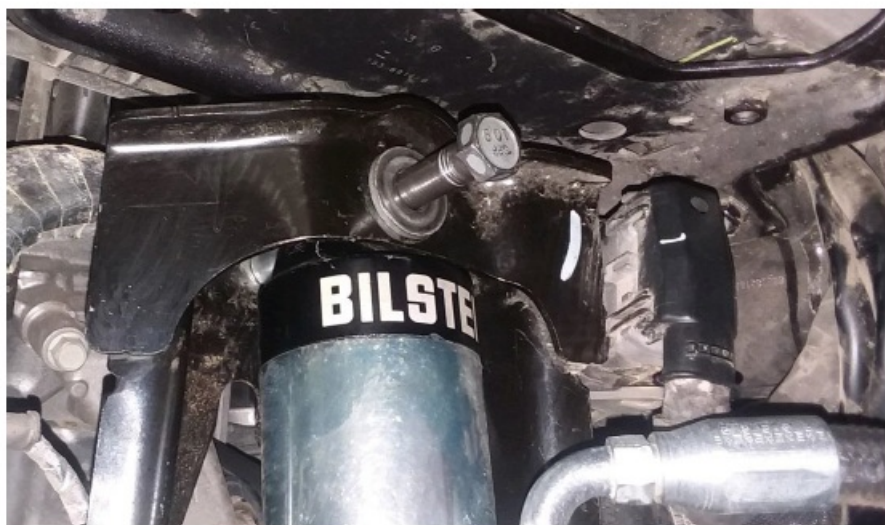
Figure 16 – Vehicle Right Side Upper Mount
