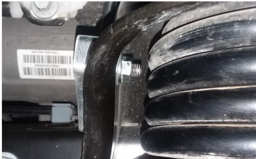
Figure 11 – Vehicle Left Side Serrated Flange Nut Installed
