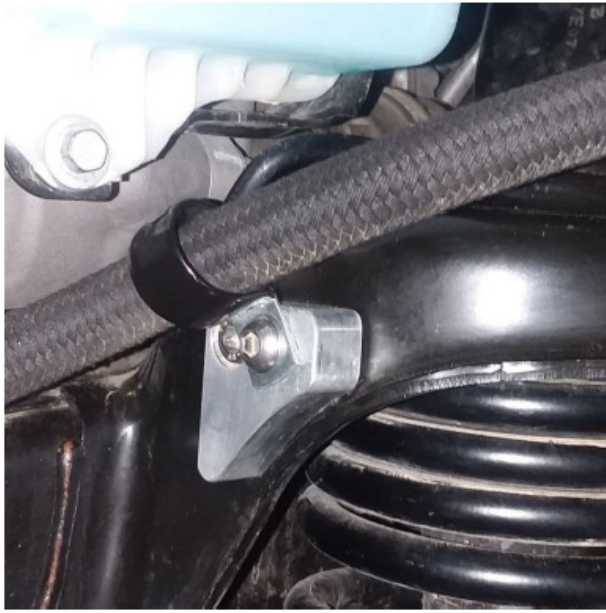
Figure 27 – Left Reservoir Hose Installed
