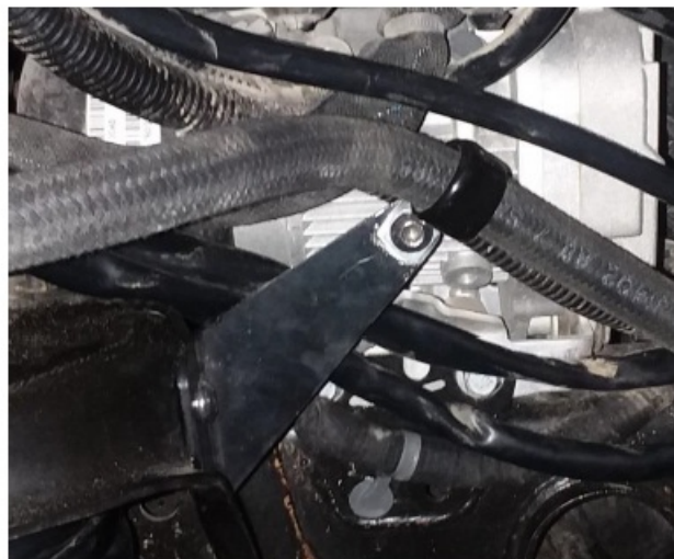
Figure 29 – Right Reservoir Hose Installed
