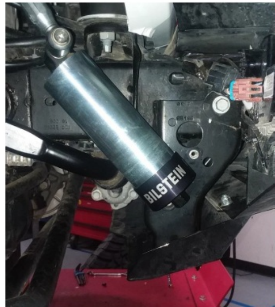
Figure 23 - Right Front Reservoir Slide Into Mount
