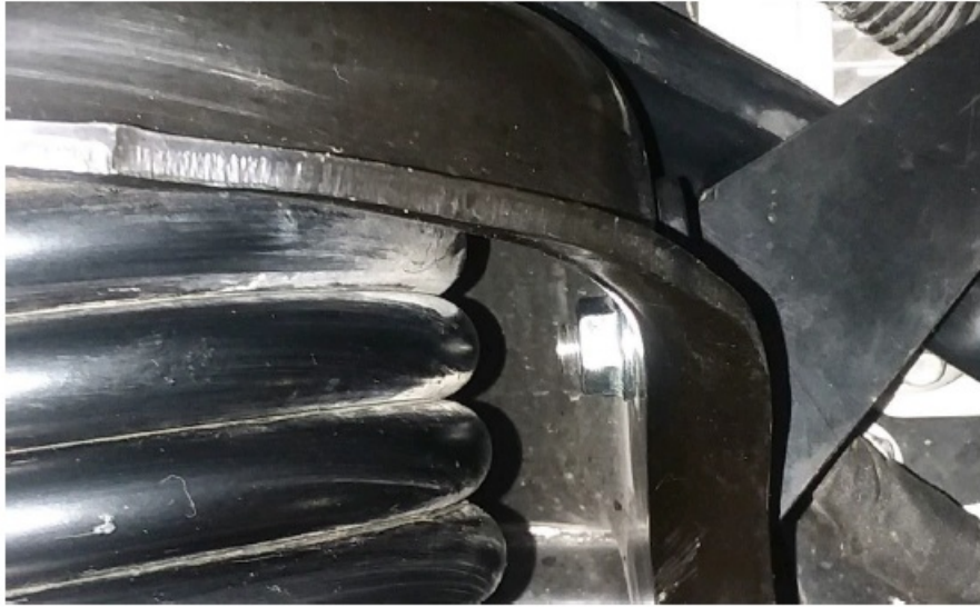
Figure 14 – Vehicle Right Side Serrated Flange Nut Installed
