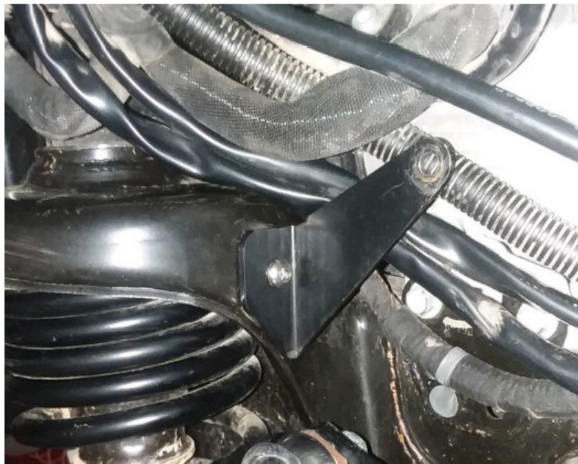
Figure 13 – Vehicle Right Side Hose Bracket
