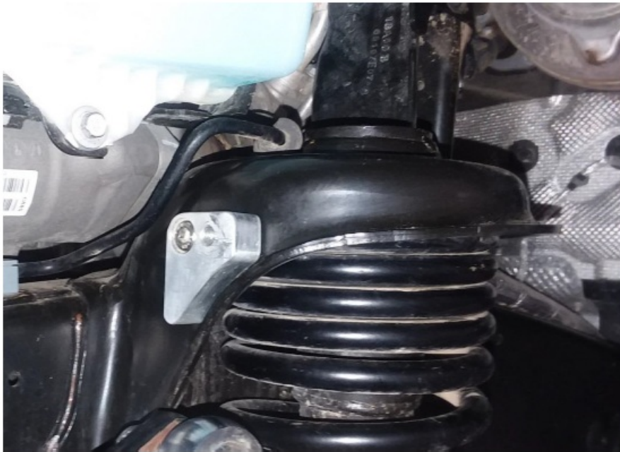
Figure 10 – Vehicle Left Side Reservoir Hose Mount Bracket
