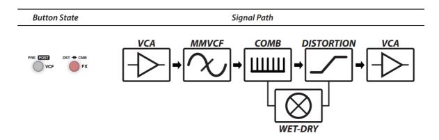
Most destructive and chaotic mode due to the nature of processing a BBD through the Distortion. Higher Input and Distortion levels may be needed to enhance these effects.
