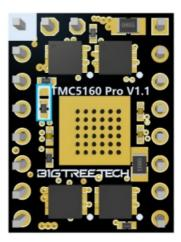
To use SD\_MODE =0, step signal is made by the internal ramp generator the resistor is welded to the other side as shown
