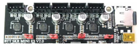
As shown in the figure, the Sensorless homing function can be used to connect the corresponding axis with the jumper cap.
