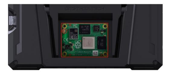
6. Cover the heatsink back onto the CM4.
