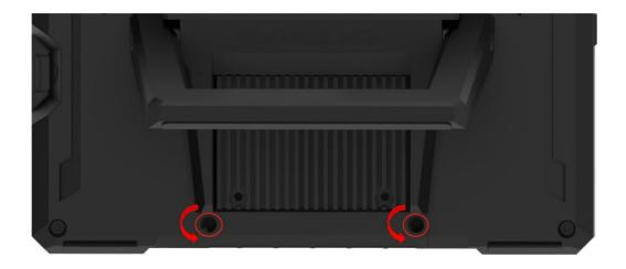
3. Use a 2.0 mm hex key to remove the four M2.5 x 10 socket head cap screws in a counterclockwise direction.
