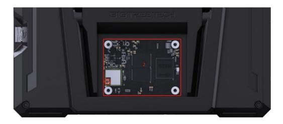
5. Align the BTB connectors of the Pad 7 and CM4.
