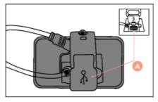
Below the display is a USB port **(A)** where you can charge, for example, your smartphone or navigation device while cycling. You must activate the port by pressing the "set" and "+" buttons for a few seconds.
