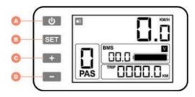
Press the "On/off" button (A) once to turn on the lights. A symbol will appear on the display. Press button (A) again to turn it off.
