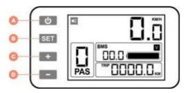
Press the "SET" button **(B)** for a few seconds, maintenance menu will appear. Press the "- "button **(D)** once to reset trip mode. Press the "SET" button **(B)** again to exit the menu.
