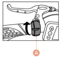
By pushing the lever (A) forward when stationary, the walk assist will be activated (which gives support up to 6 km/h). Walk assist will be activated when the (-) button is pressed for a few seconds.
