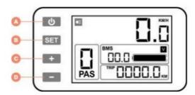
Press the "On/off" button (A) left of the display to turn the electric circuit on. The display is turned on and a menu appears.
