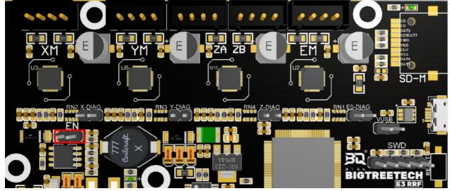
2). When using USB to power the motherboard: the jumper is inserted in the following "VUSB" position
