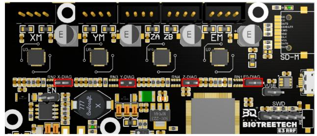
Use the jumper to connect the corresponding axis as shown in the figure to use the Sensorless homing function;
