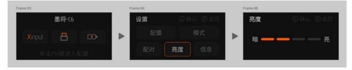
Press the left and right of the D-Pad to adjust the brightness of the backlight, there are 4 levels in tota
