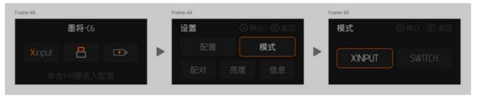
Note: To connect iOS and Android devices via Bluetooth, you must first switch to Xinput mode.
