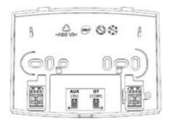
**Note:** AUX (IN) input can be connected to a free contact, with a non-polarized bipolar cable < 10 m, of auxiliary remote control devices (GSM, IoT, Home Automation, Zone, ...). Closing it allows the start of pre-established states, programs and sets that can be set via parameters. Closing it allows, only for HEATING MODE, the start of pre-established states, programs and sets that can be set via parameters. If WFC03 is connected for remote manage by APP the AUX input doesn't work.
