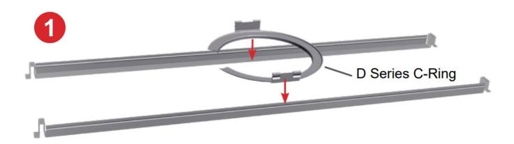
1. Place 48" tile rails with flat sides in (as shown) the appropriate distance apart and install the C-Ring. Install the ceiling tile and loudspeaker per regular installation practice. 24" rails are not needed.
