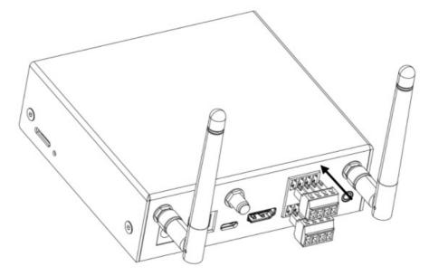
b. Installing Cable DI/DO to block terminal. Then, to use Screwdriver fix the cable.
