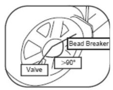
Firmly fix the wheel on the turntable clamps. (If the mounting head of the tyre changer is positioned at 12 o'clock, then the valves stem should be at the 11 o'clock position.) Apply lubricant to both tyre bead and rim, and then remove the upper tyre bead.
