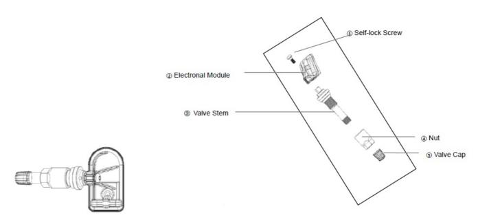
Before the transmitter is installed, the rim around the hole must be cleaned with a cloth.
