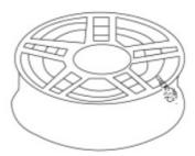
Lock the rim on the tyre changer. (If the mounting head of the tyre changer is positioned at 12 o'clock, then the valve should be at the 7 o'clock position.) Apply lubricant on both the tyre bead and rim. Mount the lower tyre bead on the rim. Ensure that the tyre bead does not touch the electronic module during mounting.
