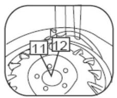
Use the same procedure to dismount the lower tyre bead. (If the mounting head of the tyre changer is at the 12 o'clock position, then the valves stem should also be at the 12 o'clock position.)
