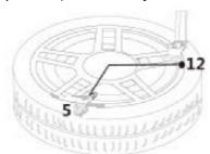
Apply soapsuds on the valve tip. If no leakage is found, put on the valve cap60. If unsuccessful, try again.
