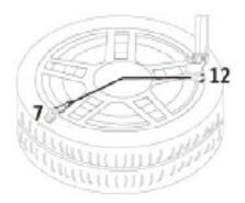
Mount the upper tyre bead the same way. (If the mounting head of the tyre changer is positioned at 12 o'clock, then the valve should be at the 5 o'clock position.) Inflate the tyre to nominal pressure.
