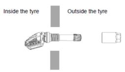
Place nut@ on the valve stem, and tighten with 5 Nm (44 inch pounds) torque.
