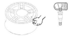
Take off the nut@, insert the valve stem through the rim hole from inside.
