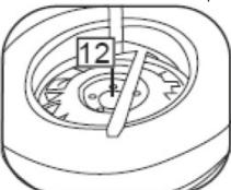
Final inspection: Visually inspect the rim, valve stem and electronic module to ensure no damage has occurred.
