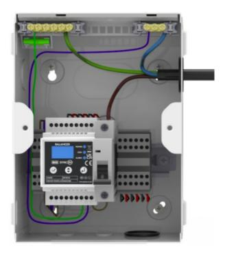
8. Terminate a twisted pair cable to the output terminals, these can be lopped in/out of each charger or multiple connections can be terminated into the Balancer. Ensuring correct polarity into the hub and the chargers. EVAB1ETP400
