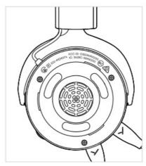
· You can remove the ear pad by turning it anti-clockwise.
