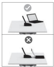
Two Classis RM 31 Q should not be directly placed back to back, because the loudspeaker of the second builtin or desktop microphone unit will be picked up by the microphone and cause feedback. The minimum distance should be 15 cm.
