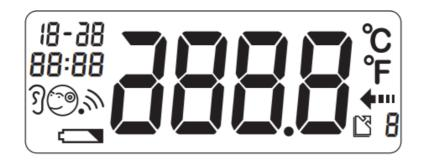
Press the U button for 1 second to switch the thermometer on. The device performs a brief self-test: all elements of the display are shown for approx. 1 second. Following a successful self-test, the device emits two short beeps. In Standby mode, the date and time are shown, and "—" is displayed.
