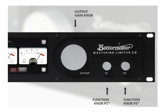
\*NOTE: both function knobs can be pressed to select various functions.
