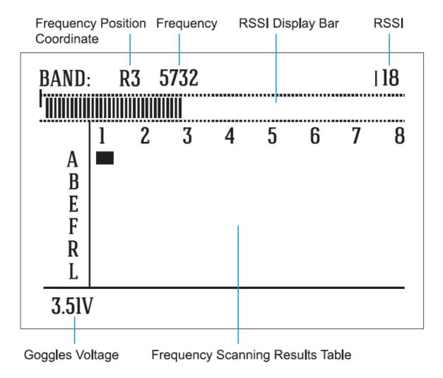
Press and hold the search button for 2 seconds to activate frequency scan, result will be displayed after 3 seconds. The different colors in the screen indicate the current status of each frequency as follows:
