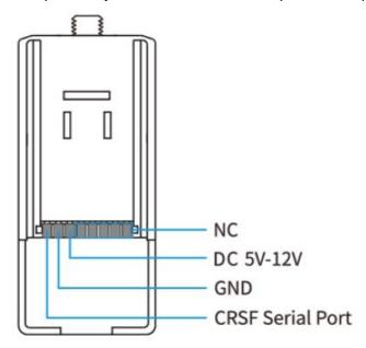
**Note:** Please assemble the antenna before power on. Otherwise, the PA chip in the Nano TX module will be damaged permanently.
