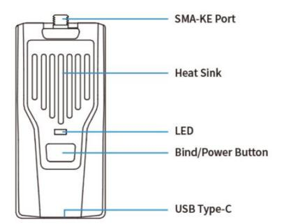
BETAFPV Nano RF module is compatible with radio transmitter which has the nano module bay (AKA lite module bay, e.g. Frsky Taranis X-Lite, Frsky Taran is X9D Lite, TBS Tango 2).
