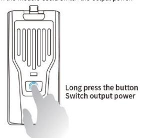
The RF TX module output power and LED indication as show below.
