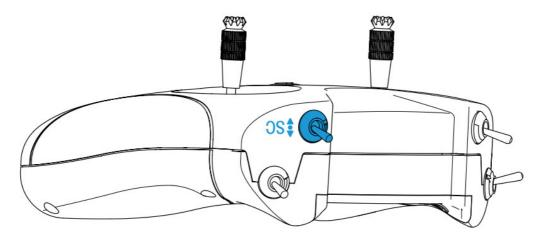
Move the Switch SC Up and Down to Change the Speed Threshold
