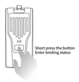
Note: The LED will NOT flash when enter binding status. The module will exit from binding status 5 seconds later auto.
