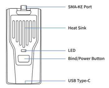
BETAFPV Nano F module is compatible with radio transmitter which has the nano module bay (AKA lite module bay, e.g. Frsky Taranis X-Lite, Frsky Taranis X9D Lite, TBS Tango 2).
