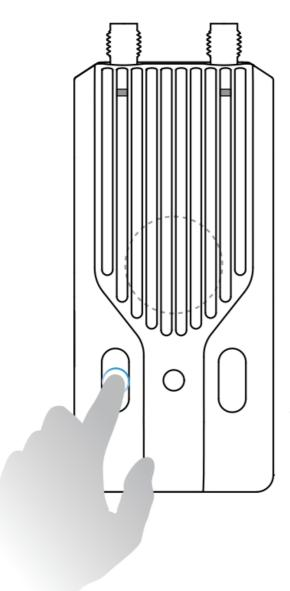
Quick Press the Key for Three Times to Enter the Binding Mode
