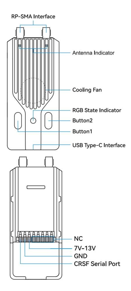
**Note:** Please assemble the antenna before power on. Otherwise, the PA chip will be damaged permanently. BETAFPV SuperG Nano TX Module is compatible with radio transmitter which has the nano TX module bay (AKA Lite module bay, e.g. BETAFPV LiteRadio 3/3 Pro, Radiomaster Zorro, Frsky Taranis X-Lite, Frsky Taranis X9D Lite, TBS Tango 2)
