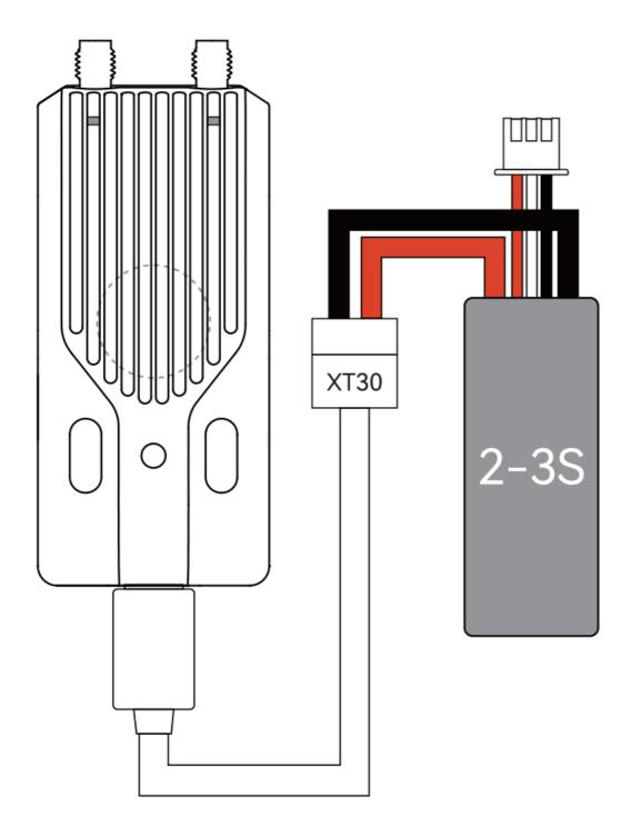
The power consumption of the module is not only related to the transmission power, but also to the telemetry ratio. For example, when the telemetry ratio is set to 1:128 in Gemini mode, the power consumption is 1 000mA@8V, while the telemetry ratio is set to 1:2, the power consumption is only half of 1:128. Therefore, when using a high-power module of 500mW or higher, ii is recommended to set the telemetry ratio higher in order to reduce power consumption and extend usage time.
