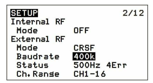
Reason: The problem is caused by the baud rate of the remote control is too low, because F1000 packet rate needs above 400K baud rate support to work.
