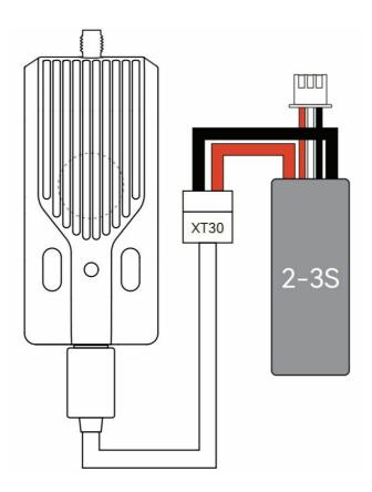
**Note:** When the voltage of the remote control battery or external battery is lower than 7V (2S) or 10.5V (3S), please do not use the 500mW and 1W, otherwise the module will be rebooted due to insufficient power supply, resulting in disconnection and loss of control.
