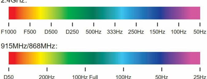
F1000 and F500 are the only packet rates in FLRC mode, only supported by ELRS 2.4G. This mode features a lower latency rate and faster configuration. However, the distance of remote control would be shorter than standard LoRa mode. It's better suitable for racing purposes.
