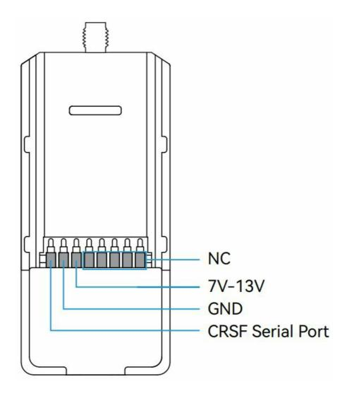
**Note:** Please assemble the antenna before powering on. Otherwise, the PA chip will be damaged permanently.
