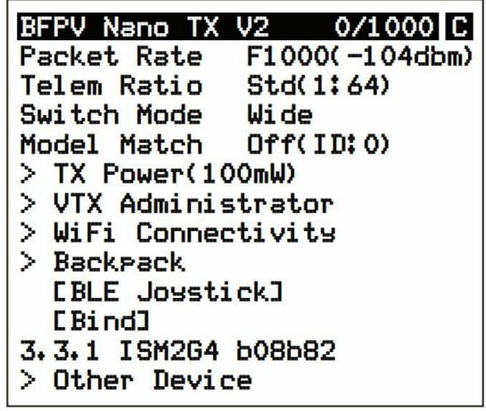
• With the Lua script, users could configure the set of parameters, such as Packet Rate, Telem Ratio, TX Power, and the like. The main functions of Lua script are shown in the table below. All function introductions can be
