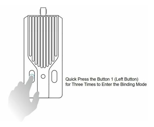
**Note:**If the transmitter module has been reflashed with a binding phrase, then using the above binding method will not be bound to other devices. Please set the same binding phrase for the receiver to perform automatic binding.
