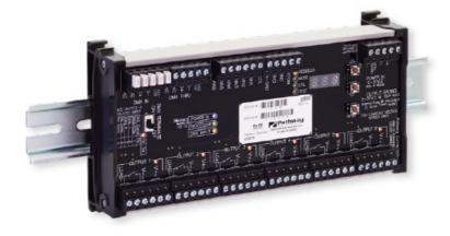
The Pathway eDIN LED Dimmer/DC Driver provides DMX512 control over LEDs and other DC devices. Each module provides 6 channels of control. When controlling LEDs, the module acts as a dimming interface only. The LED fixture will require a separate regulated DC power supply, as recommended by its manufacturer. These instructions apply to REV 2 hardware running firmware 1.6.2 or higher.
