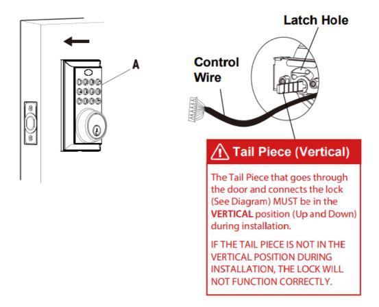
Check that the rubber gasket is secured on the exterior assembly. Insert the exterior assembly onto the door with the tailpiece going through the deadbolt latch set in the VERTICAL POSITION. Route the control wire through the door under the deadbolt latch set.
