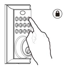
Test Unlocking Press 1-2-3-4-
