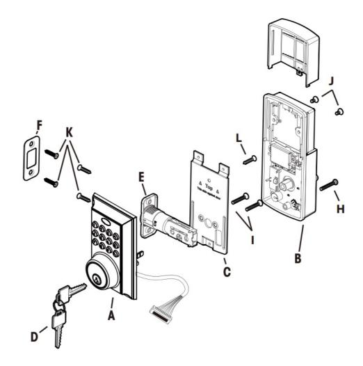
Check that the Rubber Gasket is Secured on the Exterior Assembly. Insert the Exterior Assembly onto the Door with the Tailpiece Going Through the Deadbolt Latch Set in the VERTICAL POSITION. Route the Control Wire Through the Door Under the Deadbolt Latch Set.
