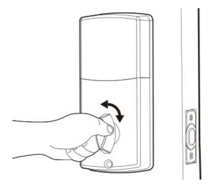
Lock/Unlock: Using the Knob to Make Sure the Latch is Extenting and Retracting Easily. If Not, Go Back to Step 2.
