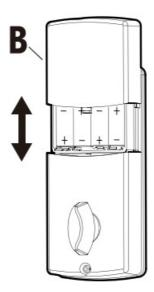
This Electronic Lock Requires (4) High Quality AA Alkaline Batteries. When All 4 Batteries are Installed in the Correct Position, You should Hear 2 Beeps and the Keypad will Illuminate Blue.
