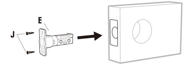
Deadbolt Latch Must Be Retracted During Installation
