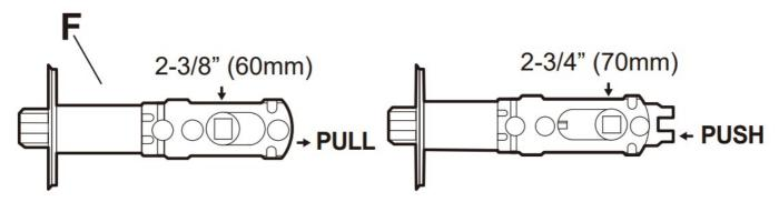
To convert between 2-3/8" (60mm) and 2-3/4" (70mm) backset 1. Pull or push the extension plate to the required size.
