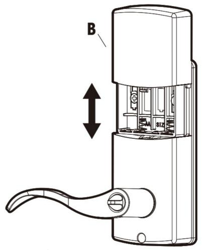
This electronic lock requires (4) High Quality AA alkaline batteries.
