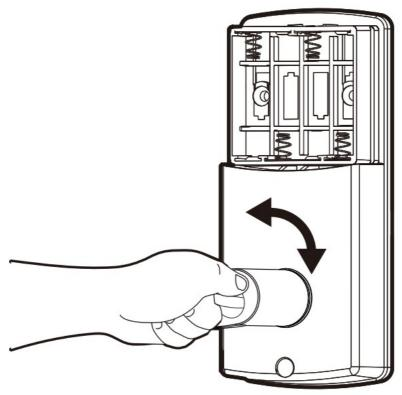
Check the Lock/Unlock function and that the Lever fully retracts the Latch.
