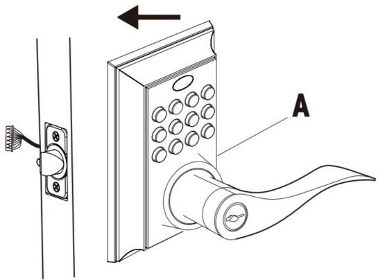
Check that the rubber gasket is secured on the exterior assembly. Place the exterior assembly onto the door with the tail piece going through the latch assembly. Route the control wire through the door over the latch assembly.
