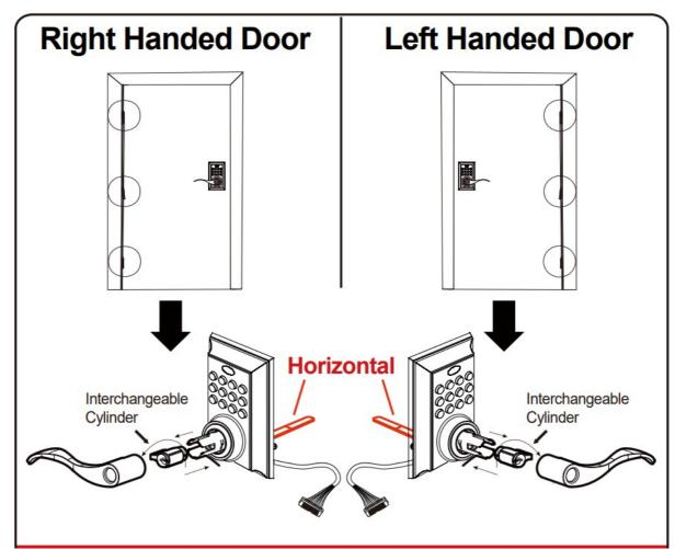
Reminder: Tail piece must be in the horizontal position only when removing or installing handles.
