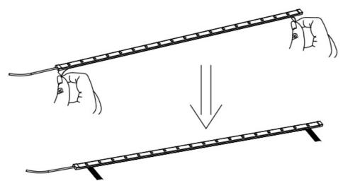
The head and tail of the LED light strip are stuck into the grooves at both ends, and the fixing parts at both ends are locked with screws.
