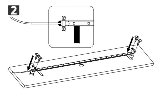
Tear off the whole protective paper, and flatten the strip light so that the LED light strip is completely adhered to the wood.
