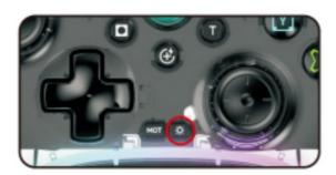
1. The button on the picture is to adjust the LED light
