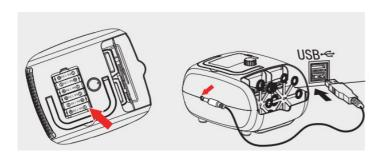
NOTE: It is recommended to remove the battery after use to prolong the use life of the machine.
