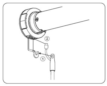
On Banded Shades, Roller Shades and Sheer Shadings, with the wand control buttons facing you, attach the top of the wand on the metal hook support (1) on the motor control side, then connect the cable into the motor head (2).
