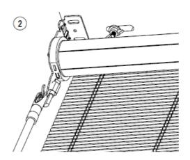
On Natural Woven Shades, with the wand control buttons facing you (1) approach the hook with the wand parallel to the headrail. (2) Gently twist the wand to attach it to the hook. Connect the cable into the motor.
