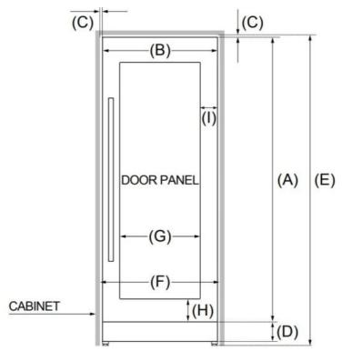
**NOTE:** The wine column comes with a 4" (100 mm) stainless steel toe kick installed to fit a standard 84" (2134 mm) tall cabinet niche.
