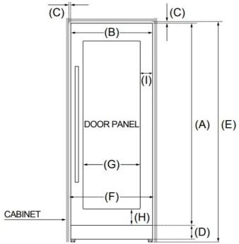
**NOTE:** The wine column comes with a 4" (100 mm) stainless steel toe kick installed to fit a standard 84" (2134 mm) tall cabinet niche. For flush installation in a standard 25" (635 mm) deep cabinet niche, maximum door panel thickness is 3/4" (19 mm).
