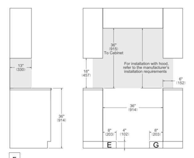
A properly-grounded horizontally mounted electrical receptacle should be installed no higher than 3" (7.6 cm) above the floor, no less than 2" (5 cm) and no more than 8" (20,3 cm) from the left side (facing product). Check all local code requirements.
