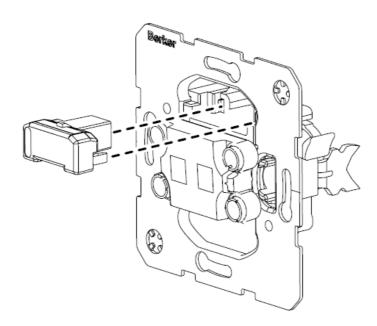
• Insert LED unit with plug-in contacts from the front into the contact sockets and press until it clicks into place.
