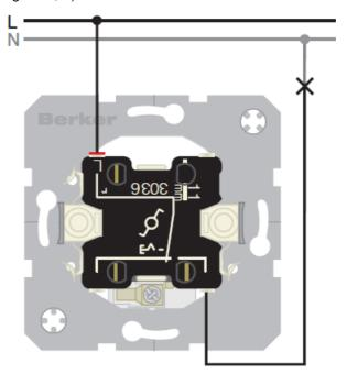
• Behind the contact bridge is the screw terminal for connecting the neutral conductor (Figure 1, 3).
