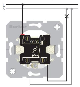
• Connect switch acc. to wiring diagram (Figure 4).
