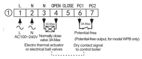
Linkage control; delay time of linkage control is adjustable
