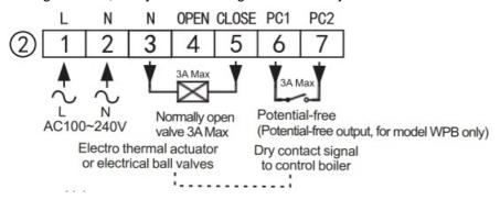
Linkage control; delay time of linkage control is adjustable
