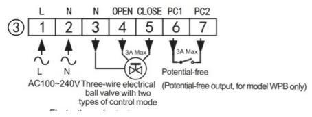
Linkage control; delay time of linkage control is adjustable
