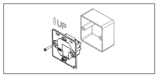
4. Re-mount the front cover via a snap-fit connection.
