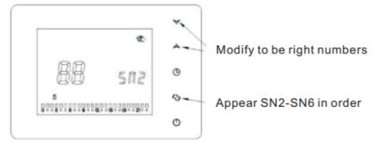
The third step, every time pressing once , it will appear SN2, SN3, SN4, SN5 and SN6 in order. Refer to second step, press Aor ▼ to modify.
