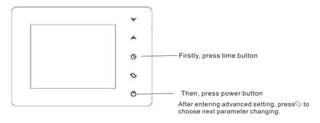
In the state of power-off, long press and hold  $\boxdot$  then press $\textcircled{\textbf{0}}$  into advanced setting mode. Then press $\textcircled{\textbf{0}}$  to set relative item.
