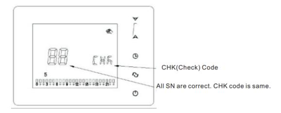
The forth step, after SN is finished setting, if CHK Code is the same with bar code, it is correct. If not consistent, it is not correct. Please input again. 3.VAC: Control valves1-8 place numbers. The default value is 01. (This setting is only useful when thermostat is applied to control Wireless Main-Control Centralized Controller. If thermostat is used to control boiler, this setting must be 01.)
