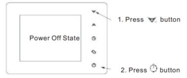
The first step, press♥ button under power off state, then press ⊕button, then press ⊕ button to enter parameter setting;
