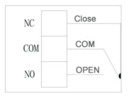
NC: Normally Closed Interface (Boiler or Loading);
