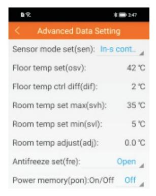
Display Code Function **Setting And Options** Factory Defult In-s control SEN Sensor mode Out-s control In-s control In-s control., Out-s limit osv Floor set temp. range 5-99℃ **42**℃ DIF Floor temp. ctrl diff 1-9℃ 2℃ Room temp set max 5-99℃ 35℃ SVH SVL 5℃ 5-99℃ Room temp set min ADJ Room temp. adjust **-5-5**℃ 0℃ Anti-frozen FRE close/open Close Power memory PON off/on On
