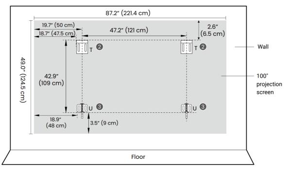
2. Use a level to ensure that the screw holes for mounting brackets (T) are aligned horizontally before drilling. Each mounting bracket (T) should be fastened by two M5 x 40 screws (V). If you might need to adjust the screen height, fix the screws to the center of slots as illustrated.
