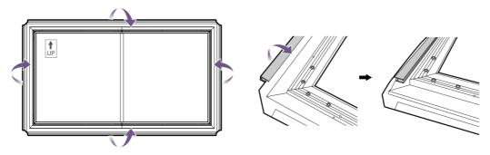
8. Fix the inner frame with the edge trim using the M4 x 60 screws (M). The screws should be fixed from the screw holes inside the frame all the way out to the nuts just inserted into the edge trims. Follow the order specified in the illustration to complete fixing 24 screws. Start from the middle of each side (as indicated by  $1 \sim 24$ ) in order to stretch the screen material properly.
