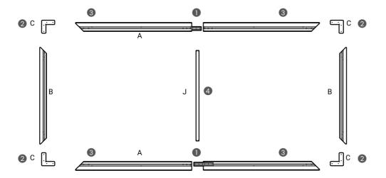
1. Connect the left and right parts of the long inner frame (A). Fasten them with three M5x10 screws (K). Complete the inner frame assembly of two long sides.
