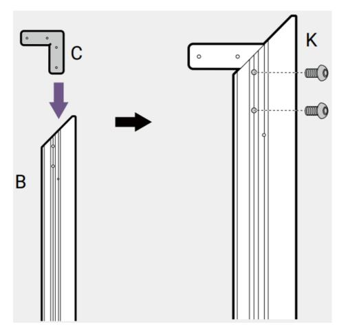
3. Align the short inner frame (B) with the brackets (C) on both ends to the long inner frames (A) together. Fasten them together with M5 x 10 screws (K). Follow the illustrations to install the other short side and make the inner frame a square.
