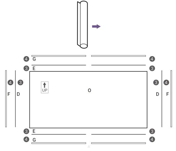
3. Insert the fiberglass rods (D & E) through the openings on the screen material edges. Follow the illustration to complete the long and the short sides.
