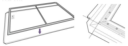
6. Insert nuts (N) to the edge trims as illustrated. Insert the number of nuts to each side as specified in the illustration. That will be 8 nuts on each long side, and 4 nuts on each short side. Slide the nuts evenly to align with the screw holes inside each inner frame as illustrated by the circles.
