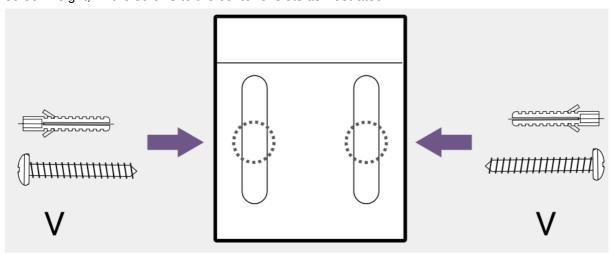
3. Use a level to ensure that the screw holes for spring screws (U) are aligned horizontally before drilling. Each spring screw (U) should be fastened by two M5 x 40 screws (V) screws. If you might need to adjust the height, fix the screws to the center of slots as illustrated
