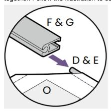
5. While the screen material is still placed and facing downwards on the floor, place the assembled inner frame gently on top of the screen material. Adjust the edge trims (F & G) so they are alighted with the inner frame on the same side.
