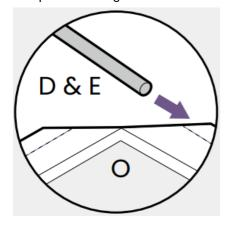
4. Snap the edge trims (F & G) to the screen material edges to hold the screen material and the fiberglass rods together. Follow the illustration to complete the long and the short sides.
