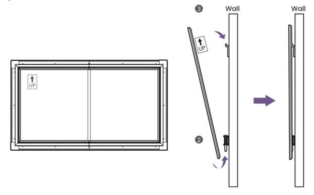
4. Check if the screen is mounted properly. Hold the screen from both sides and slide it up and down gently. If it is stable, the screen mounting is complete.
