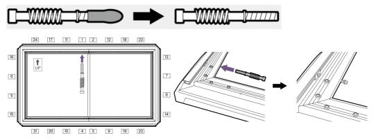
9. Lift the screen material and the frame carefully without touching the screen surface. Check if the screen material is properly stretched. To adjust the stretch, work from the screws. Once the adjustment is done, lay down the screen gently facing downward again (with the protection of the supplied nonwoven sheet). Secure all screws.
