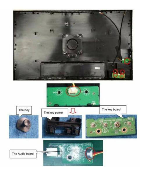
**Note:** The positions of the clips on the rear cover are as follow. There are some small gaps between CLIPS. It's su,.9gested to separate bezel and rear cover from th aps.
