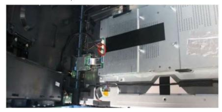
Remove the screws and disconnect the connectors to remove the Key board and ~he Audio board.
