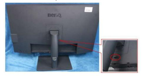
Remove the screw to remove the stand assy and the base assy.
