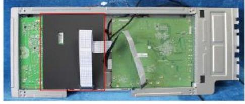
And then remove screws in red, pull out the wire to remove the mainboard and power board.
