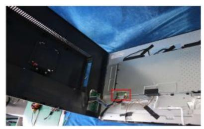
Unscrew the screws and disconnect the connectors to remove the USB board,
