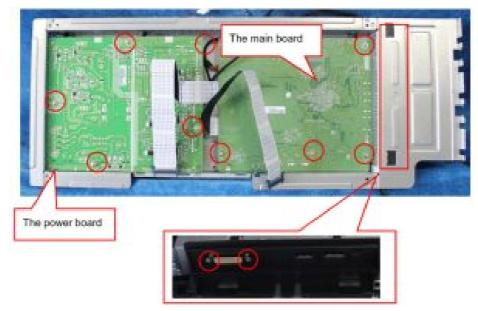
Turn over the power board and mainboard; remove the cables.
