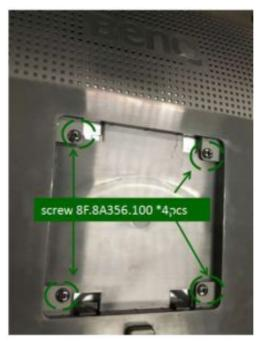
2. Remove Slider module from RC by Screwdriver and hand
