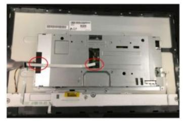
2. Remove LVDS from PANEL, and remove the screw by screwdriver
