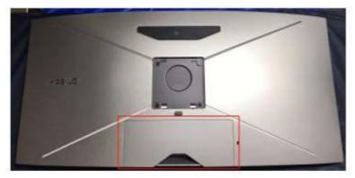
2. Release the screws and use the tool (not provided) to open all the latches slowly and carefully from the bottom side of back cover.
