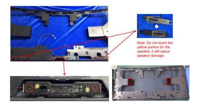
Take out the bezel from the panel, then remove the HDR keyboard from the bezel by releasing the screw.
