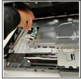
Disassemble SPK Wire connector
