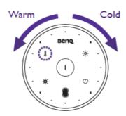
Tap the Color Temperature Adjustment button to activate color temperature control. The indicator will light up when the color temperature control is on. Rotate the adjustment ring to adjust the color temperature and the lights around the adjustment ring will change accordingly. Rotate the adjustment ring clockwise to increase the color temperature (the highest color temperature is 6500K), or counterclockwise to decrease the color temperature (the
