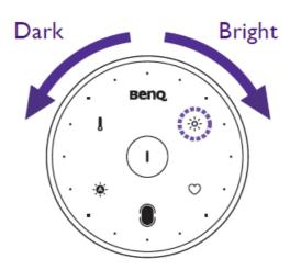
Tap the Brightness Adjustment button to activate brightness control. The indicator will light up when the brightness control is on. Rotate the adjustment ring to adjust the brightness and the lights around the adjustment ring will change accordingly. Rotate the adjustment ring clockwise to increase the brightness, or counterclockwise to decrease the brightness.
