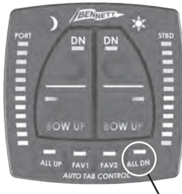
Fully Deploys (Lowers) Both Tabs
