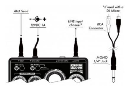
Delay/echo FX unit created as musical instrument for live improvisation. DSP audio delay, multiplied, divided and modulated in real time by dedicated controls. The unit also features analog overdrive and filters to shape delay tone and feedback.
